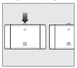
■ Press the button on the top of the salt reservoir in the direction of the arrow. The cover will pop open.
